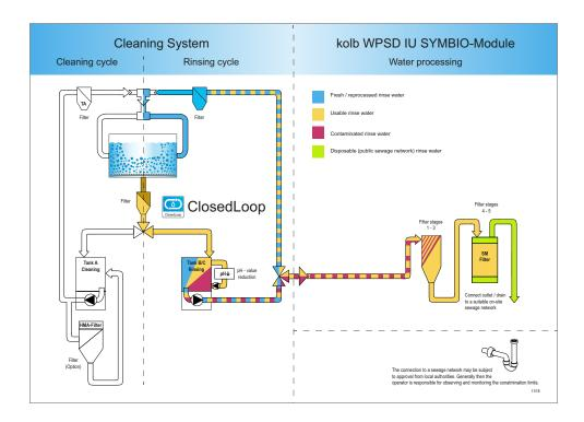
The filter stages of the WPSD IU SYMBIO-module are adapted to the rinse water to be treated and adjusted to the process. Rinse water of the upstream cleaning system that is no longer usable is either lowered to the appropriate pH value in the rinsing tank, or pumped directly into the WPSD IU SYMBIO module.
