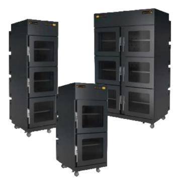
Baking Dry Cabinets from 70 Series are designed to stabilize from  $+40^{\circ}$ C to  $+70^{\circ}$ C, at RH  $\leq 1\%$ , without adjustment, in accordance with the recommendations of the J-STD-033D standard, applicable to humidity sensitive SMD components (MSL 2 to 6).
