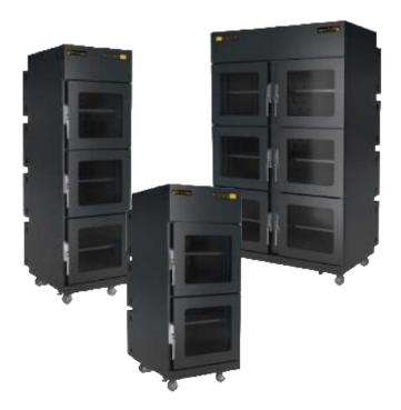
Baking Dry Cabinets from 50 Series are designed to stabilize from  $+40^{\circ}$ C to  $+50^{\circ}$ C, at RH  $\leq 1\%$ , without adjustment, in accordance with the recommendations of the J-STD-033D standard, applicable to humidity sensitive SMD components (MSL 2 to 6).
