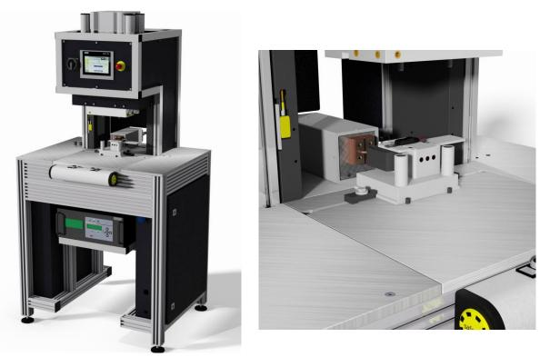
With the induction option it is possible to realize adhesion also on metallic components in one stable process step.
