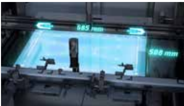
Safe processing of XL assemblies measuring up to 685 x 508 mm
