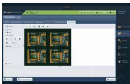
Autorouting on a PCB panel
