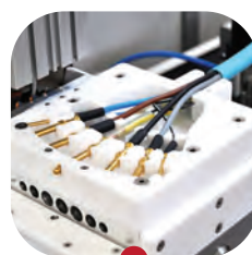
Fixtures designed in accordance with the application, ensuring a strict positioning of the shrink tube during the process
