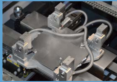
Fluxer unit with 4 spray heads
