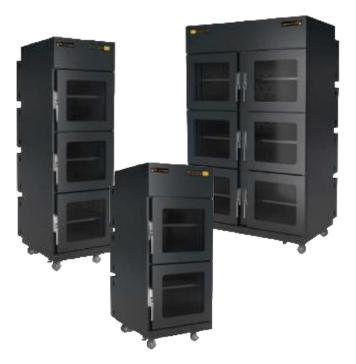
Baking Dry Cabinets from 60 Series are designed to stabilize from  $+40^{\circ}$ C to  $+60^{\circ}$ C, at RH  $\leq 1\%$ , without adjustment, in accordance with the recommendations of the J-STD-033D standard, applicable to humidity sensitive SMD components (MSL 2 to 6).
