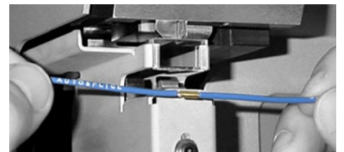
Protective guards keep operator hands away from splice tooling.
