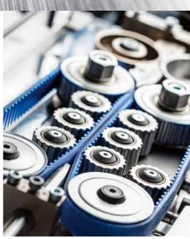
The efficient belt drive reliably draws in the cable at a speed of up to 9 m/s.
