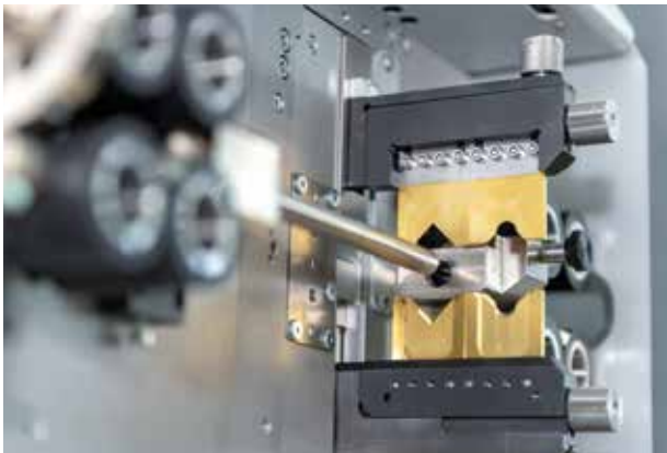
▲ Kappa 330 Double-blade principle
