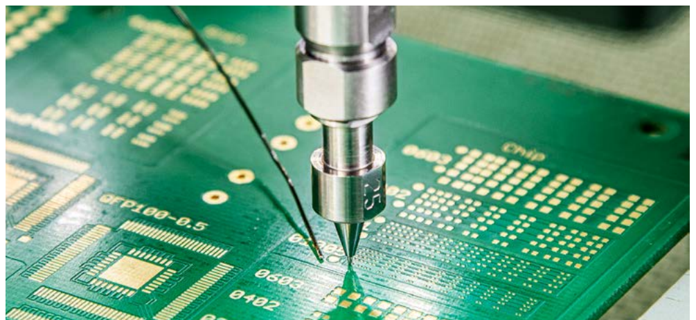
Placement of a 01005 component.
