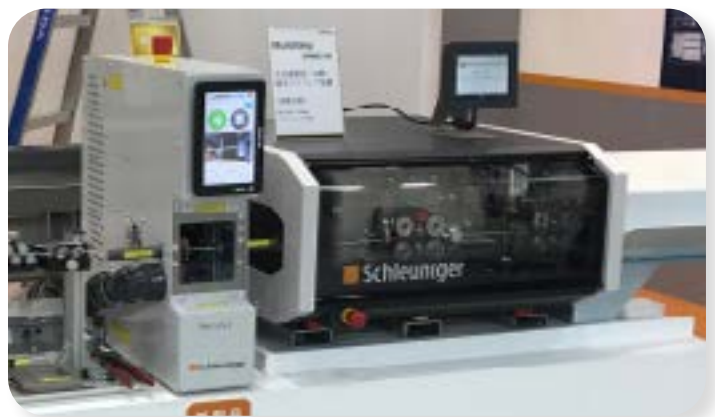
Mercury-4 in-line fixture with Schleuniger MultiStrip 9480. Also compatible with other brands/models.
