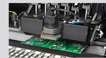
Fiducial Camera (2D) For Board Barcode Scanning
