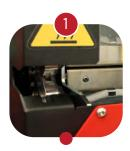
Holding system that preserves the integrity of the cable, ensuring it does not move during the entire process
