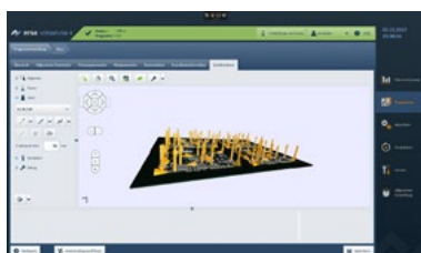
Graphical presentation of the soldering path in 3D
