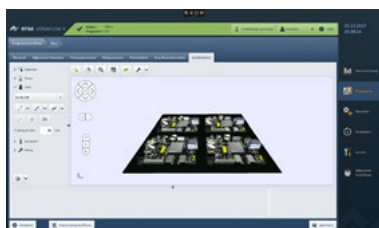
Autorouting divides the program optimal over the different solder pots
