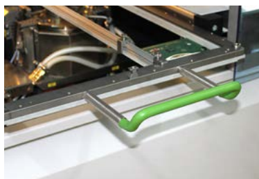
Convenient manual infeed + barcode scanner for automatic product identification
