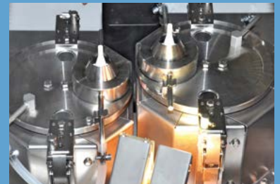
Solder module with two solder baths on the same axis
