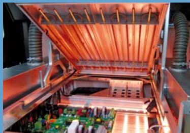
Dynamic preheating concept with top- and bottom-side heating
