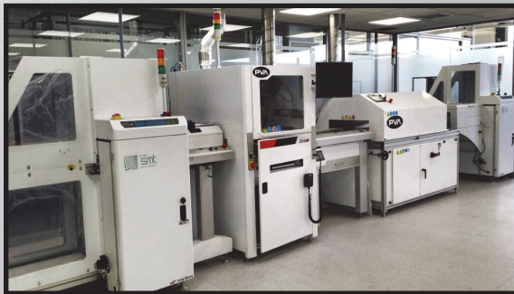
Automation installation in a PVA coating line
