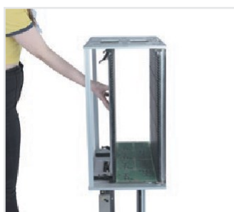
2 Slide the movable side towards the PCB until it cannot slide any further
