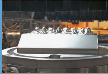
MINI-VARIO-WAVE solder nozzle for optimized throughput
