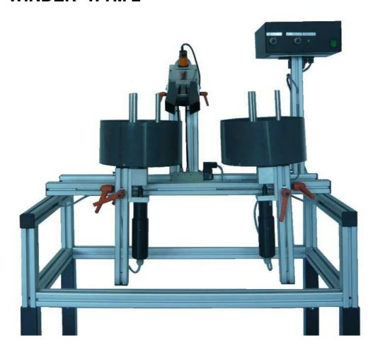
With this double pot-winder, it is possible to coil certain cables and wires to coils. The double pot-winder is available in two versions without motors and with motors. The pot winder is used behind our ISOMAT and Autocut. An installed feeder tube switches over from one pot to the other once one cable is feeded into the pot.
