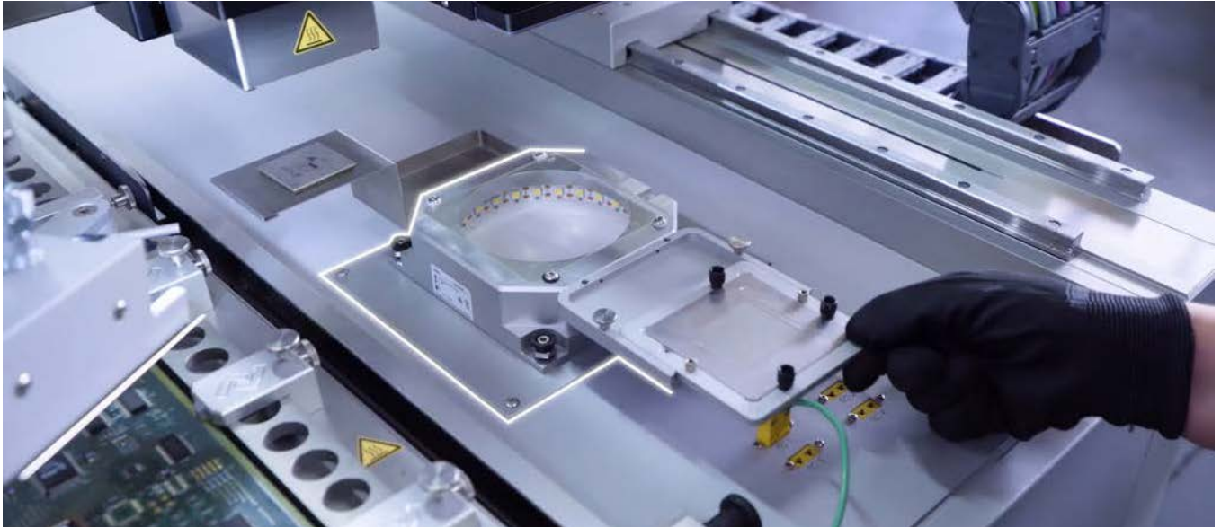
Dip&Print Station of the HR 600 XL – application of a defined amount of flux on BGA components
