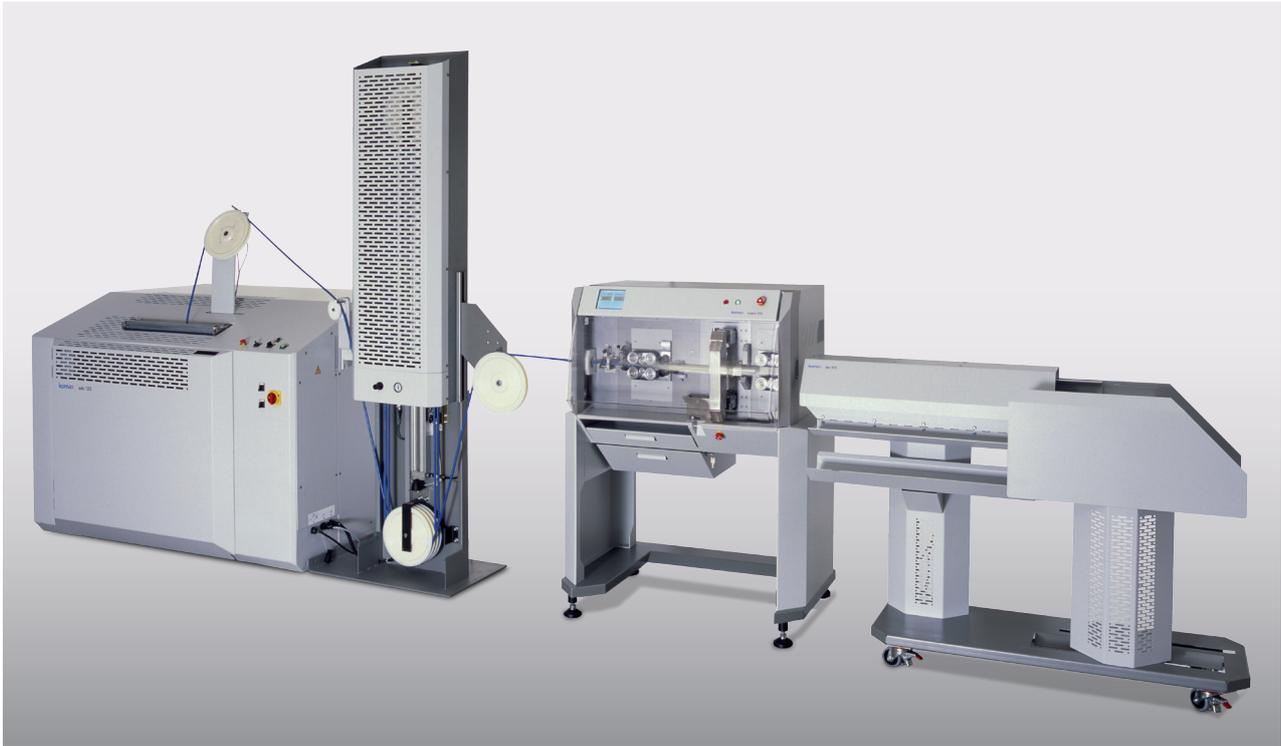
▲ **Production line** with Kappa 350 and Komax dps 375 deposit system
