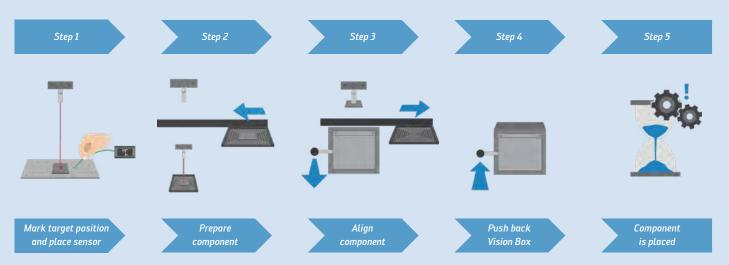
HRSoft 2 – User guidance via pictograms showing component placement as example
