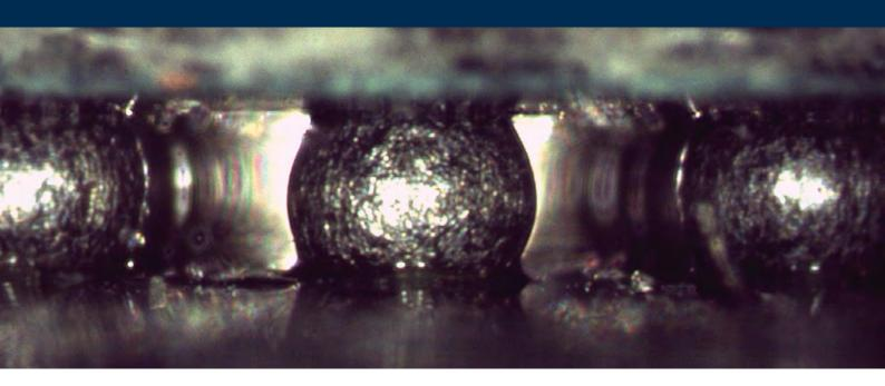
Hidden solder joint inspection is one of the most important areas in a quality assurance program. The images shown on these pages underscore the flexibility of the ERSASCOPE inspection systems.
