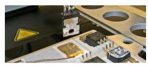
T0220 on aluminium carrier with hybrid rework system
