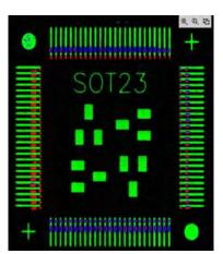
Computer-supported alignment of a QFP
