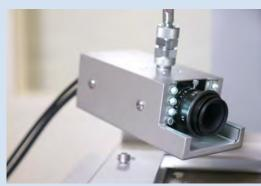
Reflow process camera on the HR 550
