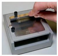
Flux deposition in the dip stencil
