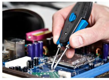
Extremely handy, precise and powerful – the CHIP TOOL VARIO desoldering tweezers
