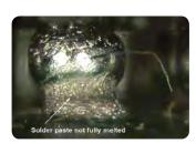
PBGA – scaling: insufficient heat
