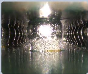
The image process function "Best Focus" enables the ERSASCOPE user to easily find the objectively best sharpness setting for any freely determined portion of the image. This is an especially useful feature when measurements are to be taken within the image.
