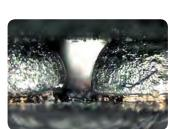
PBGA – scaling: insufficient heat
