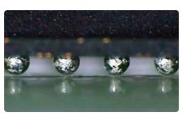
Real-time rework process visualization of BGA during
