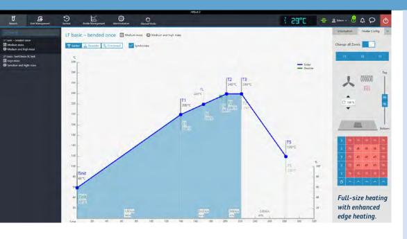
The user interface of HRSoft 2 sets new standards in rework, both technologically and optically. Being a clearly structured software platform for current and future systems, it offers the user all functions of the respective system and guides him through the single steps of the rework process.
