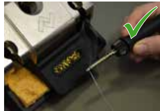
Add new solder after cleaning
