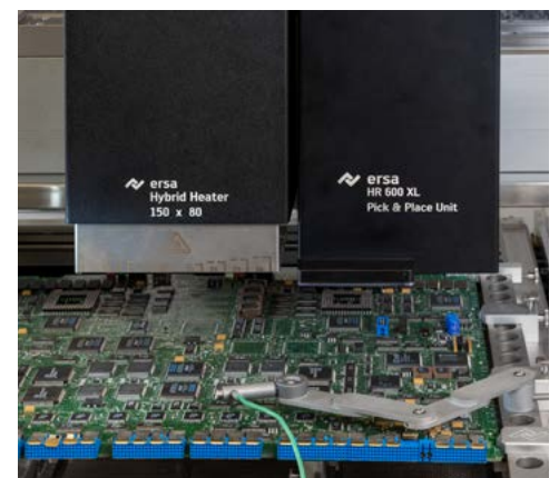
Optional extra large hybrid heater with 150 x 80 mm
