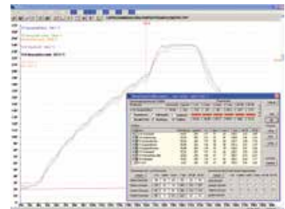
Automatic process evaluation with 6 parameters - display of gradients with up to 17 profiles
