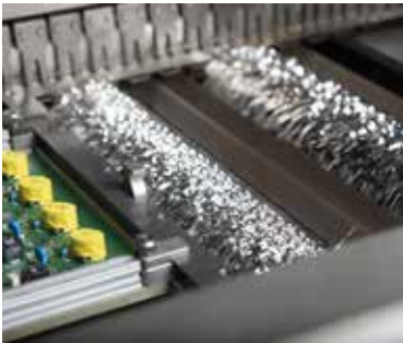
Proven Ersas dual wave soldering technology
