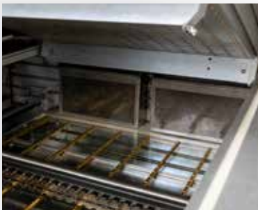
View of the preheating zone of the SMART ELEMENTS® cassettes, which are attached to the side of the efficient Erska process gas cleaning system.
