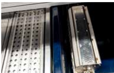
Soldering module: Proven Ersapot technology with a filling volume of only 345 kg
