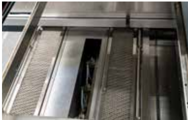
Precise spray fluxer for reliable flux application
