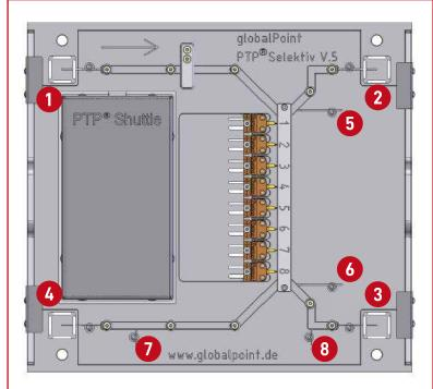
For the basic oven check-up should preferably be used all thermocouples 1 to 8. The measurement of the preheating profile of a selective soldering machine is done with thermocouples 1, 2, 3 and 4. It is recommended to determine the solder temperature with sensors 5 to 8. The contact time for a correct measurement should be  $\geq$  2 seconds.
