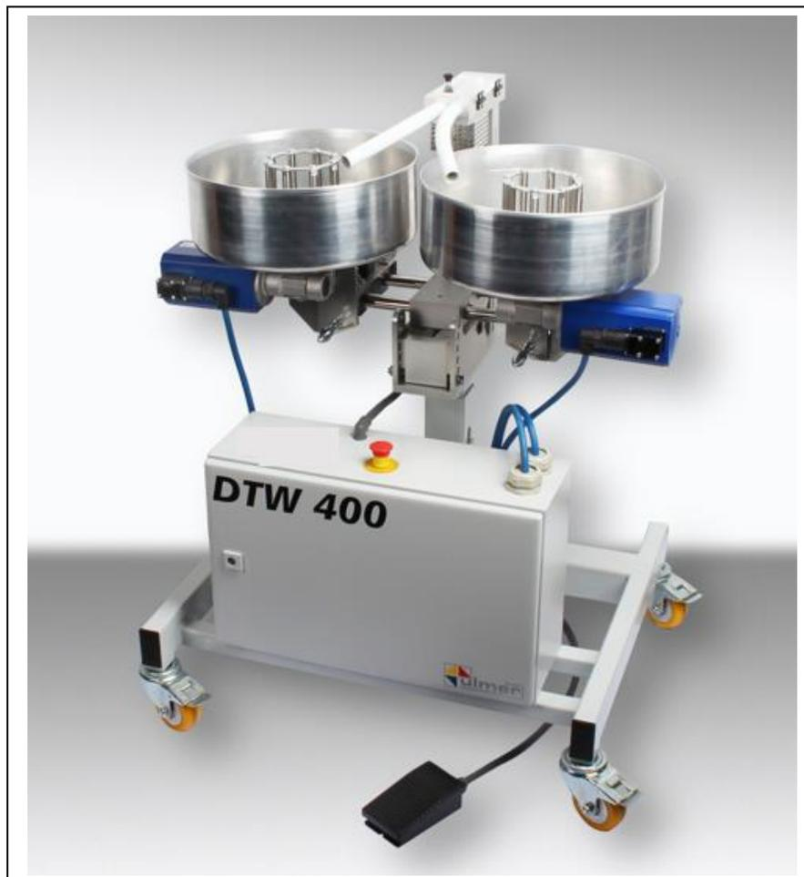
Motor-driven upwindert that is adjusted to a cutting machine SM15 2PT or a stripping machine Komax Kappa 3xx. The line from the above machine is fed to the DTW400 through an inlet channel with a separating switch. The winder is suitable for flexible cables and wires with an outer diameter of 2.0 to 18.0mm, with a minimum length of 2000mm. The maximum wrap weight must not exceed 10kg!
